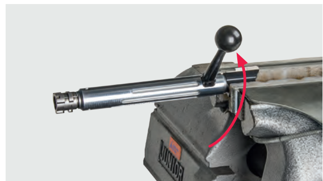
Fig. 21 Turning the bolt to uncock it
