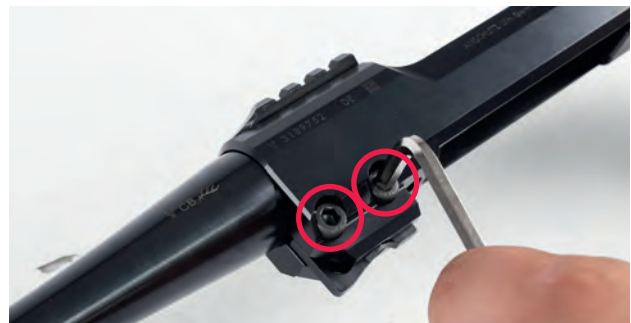
Fig. 55 Unscrewing the pivot screws
