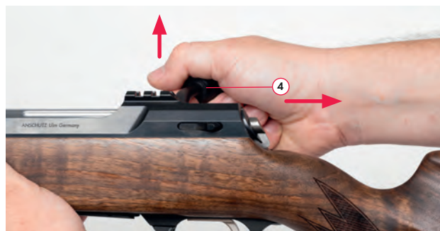
Fig. 16 Lifting the bolt handle
