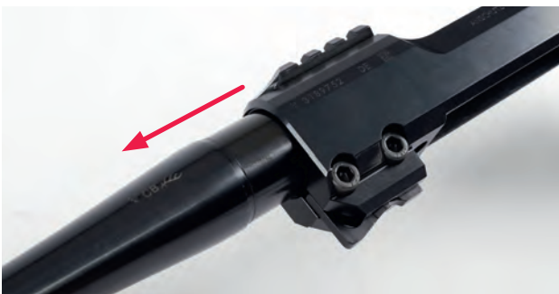
Fig. 57 Removing the barrel
