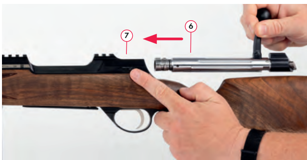
Fig. 14 Inserting the bolt
