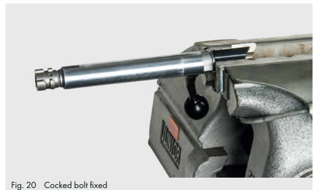
Fig. 20 Cocked bolt fixed
