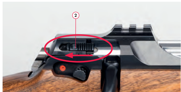
Fig. 28 Bolt handle lock activated, push to the rear to deactivate
