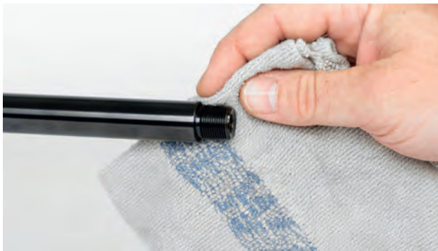
Fig. 52 Cleaning the threads
