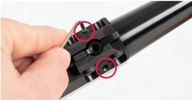
Fig. 56 Loosen countersunk screws
