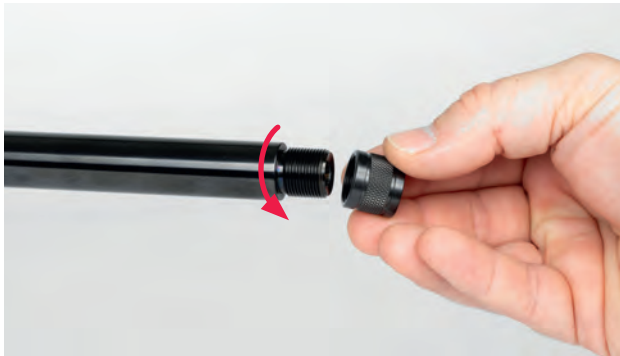
Fig. 51 Unscrewing the threaded bushing from the barrel thread
