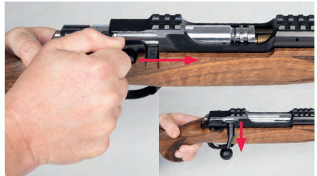
Fig. 34 Closing the bolt
