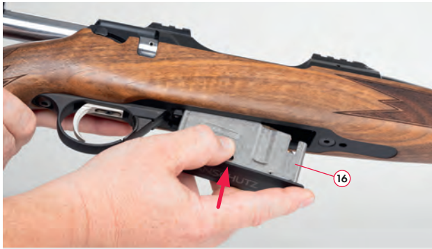
Fig. 33 Inserting the magazine
