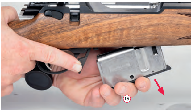
Fig. 38 Removing the magazine
