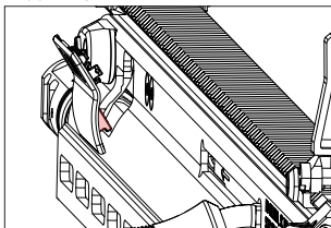
Hooking the heat shield.
