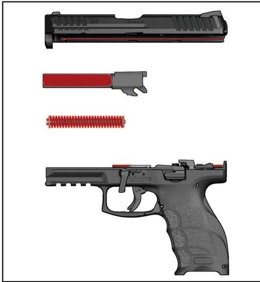
Figure 37 – Lubrications Points (in red)
