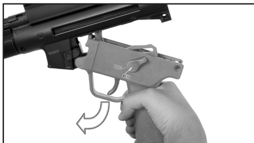
Fig. 36 – Remove pistol grip
