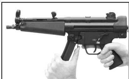
Fig. 33 – Depress the SP5 magazine release lever or button.
