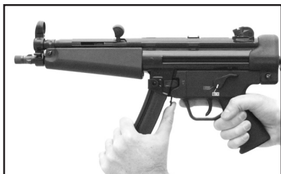
Fig. 23 – Depress the SP5 magazine release lever or button.
