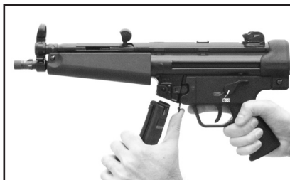
Fig. 24 – Remove the magazine from the magazine well.
